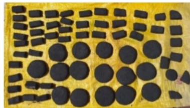
Figure 4. Printing and drying walnut shell briquettes
