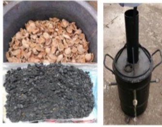
Figure 1. The process of making walnut shell charcoal
