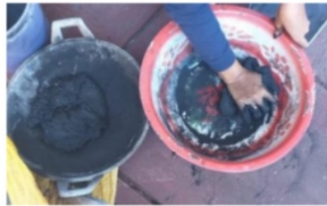
Figure 3. The process of mixing charcoal powder and adhesives
