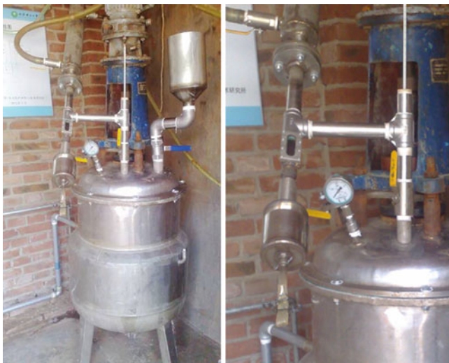
Fig. 5.8 Facilities of producing n -butyl nitrate. Left nitration reactor, right segregator with a glass mirror
