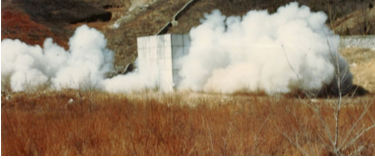
Fig. 2.45 Explosion of liquid explosives in semiclosed space
