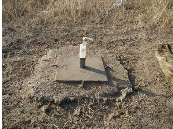
Fig. 2.26 Setup for brisance measurement of liquid explosives
