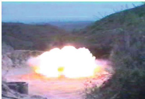
Fig. 2.32 Explosion of XJ-1 explosive (200 kg)
