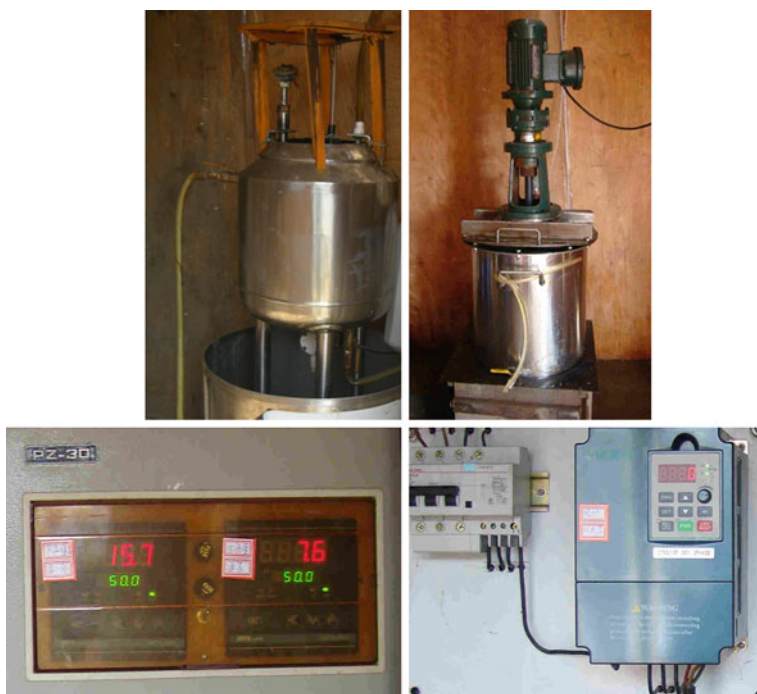
Fig. 5.11 Facilities and control systems of preparation of diethylene glycol dinitrate. 1 Open nitration reactor, 2 stability treatment vessel, 3 temperature-controlled meter, 4 frequency variator
