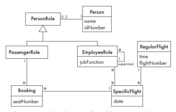
Figure 5.3 l Airline system class diagram after adding a generalization
