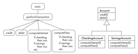
Figure 2.1 Organizing a system according to the procedural paradigm (left) or the objectoriented paradigm (right). The UML notation used in the right-hand diagram will be discussed in more detail later
