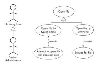
Figure 4.4 Extension, generalization and inclusion in a use case diagram
