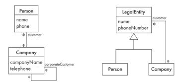
Figure 5.30 Creating a generalization of two classes which have similar features, but the names of the features are different. The left diagram is the original version; the right diagram is the improved version
