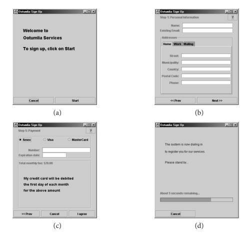
Figure 7.3 Views of the ISP sign-up application that has improvements compared with Figure 7.2 . It uses a 'wizard' approach as well as tabbed dialogs
