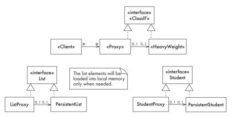
Figure 6.13 Template and examples of the Proxy design pattern
