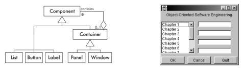
Component classes whose instances form a hierarchy in a user interface. The example shows a frame, composed of a label (top), a list (left) and two panels. The first panel (on the right) is in turn composed of four text fields. The other panel (at the bottom) contains three buttons
