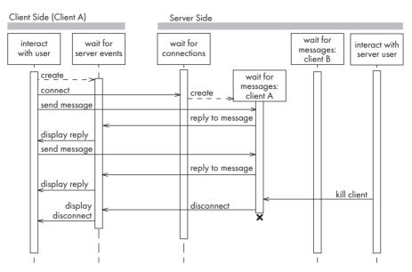
Figure 3.5 Threads in a client–server system
