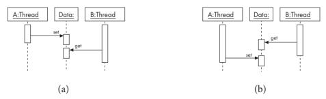
Figure 10.6 A critical race situation caused by a change in speed of execution
