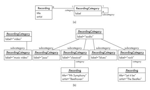
**Figure 5.12** (a) Modeling a taxonomy of products using a single class, and (b) an object diagram generated from this
