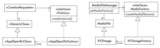
**Figure 6.14** Template and example of the Factory design pattern
