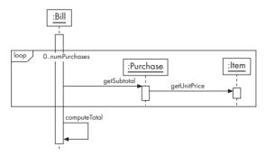
Figure 8.5 A sequence diagram showing a loop fragment
