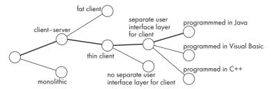
Figure 9.1 Part of a design space, showing alternative designs resulting from different choices when making design decisions. The lines represent options; the bold path is the set of decisions made
