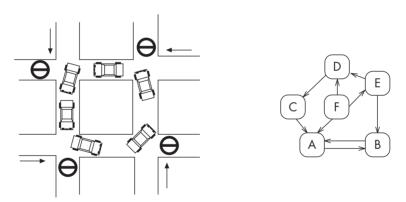
Figure 10.5 Livelock in traffic (left) and software (right)
