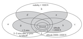
Figure 10.2 Venn diagram, with shading showing situations where the landing gear must be down, and hence the alarm must sound if it is not down. Conversely, the alarm should never sound in the unshaded areas
