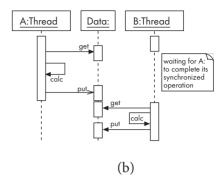
Figure 10.7 A critical race situation caused by a second thread unexpectedly accessing nonsynchronized data
