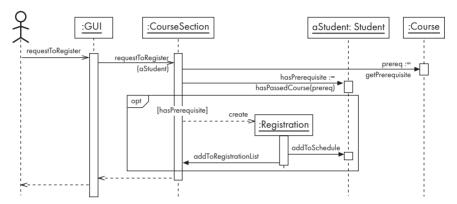
**Figure 8.4** A sequence diagram showing more detail about the student registration process including an optional combined fragment
