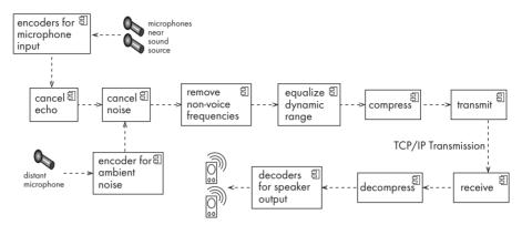
Figure 9.12 A pipe-and-filter architecture for sound processing
