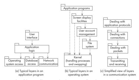
**Figure 9.3** Examples of the use of layers. Higher layers can call on the services of lower layers, but not the other way around
